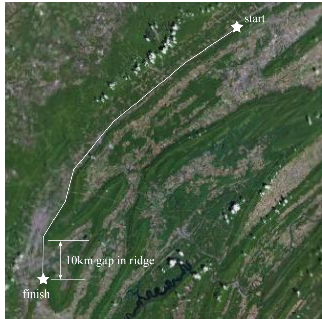
Figure 7. Altoona Gap. The flight follows the Bald Eagle Ridge from Julian, PA to Altoona, PA. In the simplified case described in the text, ridge height is 200m and it is approximately 60km to the gap. The flight ends when the gap is crossed and the ridge is reacquired.
