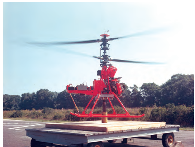
A DSN-1 (QH-50A) on a hover fixture at Gyrodyne in 1965.
