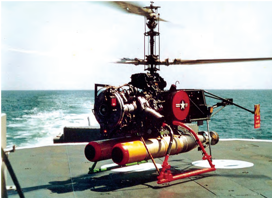
QH-50C, loaded with Mark 44 Warshot torpedoes, lifting off from a destroyer deck.
