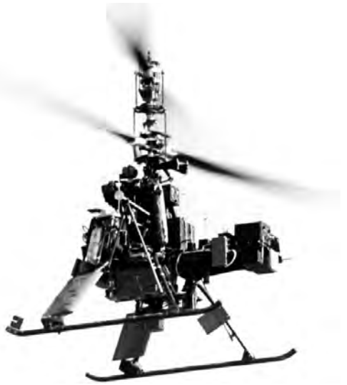
The DSN-1 (later QH-50A) was an unmanned version of the YRON-1. First unmanned shipboard landing was on December 7, 1960.
