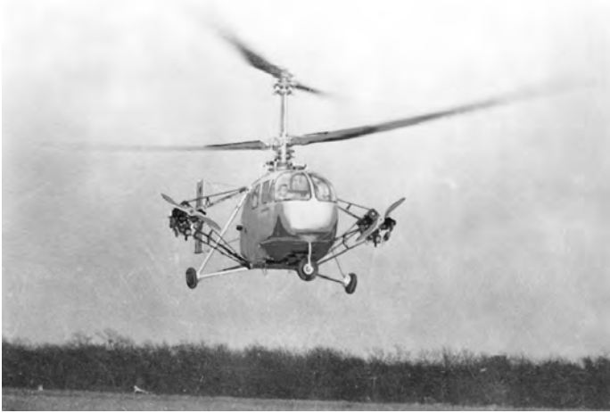
The Gyrodyne GCA-2B was the first US compound helicopter.
