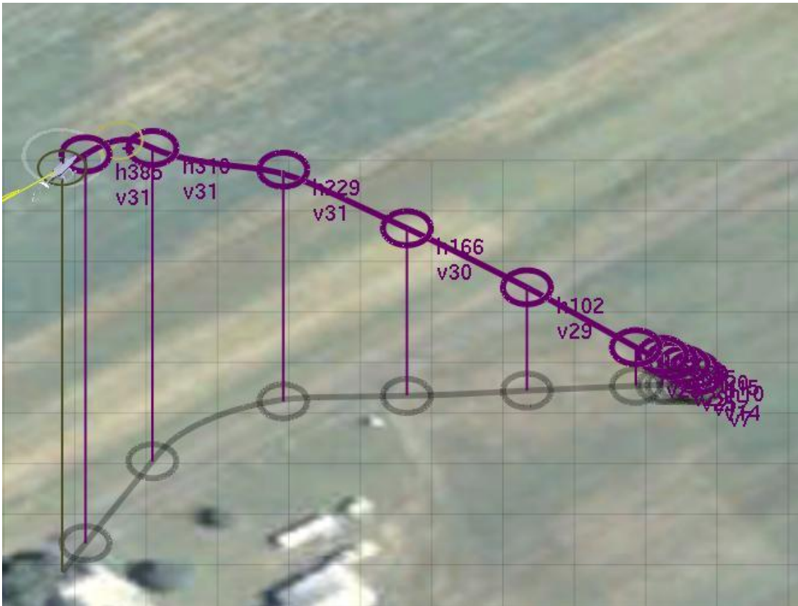
Figure 5-6. Flight path of autorotation landing flight in ground control station interface for case 2
