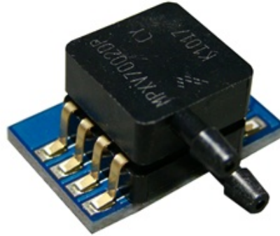
Figure 3.4. Freescale MPX7002DP differential pressure sensor [39].
