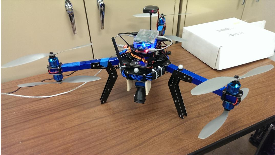
Figure 5.1: The Y6 hexacopter carrying the Odroid and Machine Vision camera used to test the system presented in this thesis.
