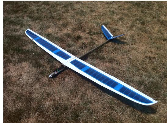
(b) Omega II motor glider (2.0 meter wingspan).
