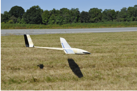
(a) RnR products SB-XC sailplane modified with an electric motor.
