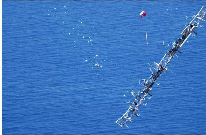
Figure 1.2: Mid-air disintegration of the Helios solar aircraft. The need for atmospheric pseudosatellite aircraft to be extremely lightweight makes them very fragile and susceptible to damage from turbulence at low altitudes. Reproduced from Noll et al. (2004) “Investigation of the Helios Prototype Aircraft Mishap; Volume I: Mishap Report” [4].
